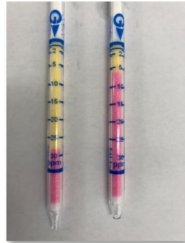
Measurement of Ammonia Concentration by the detection tube
